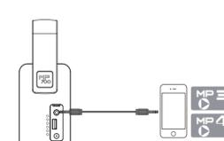
Connect to source using 3.5mm auxiliary cable included.
