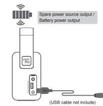
The USB output can be used to charge your mobile device up to 5V maximum 500mA DC using a USB cable. USB cable not included.
